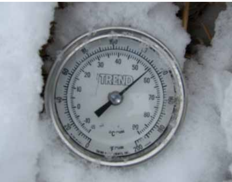
Figure 4. Temperature measurement of an end-of-lay windrow compost pile in the winter using a 3 ft probe
