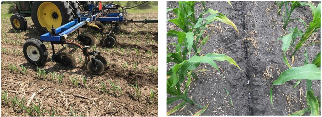
Figure 4 and 5. Ammonia slot sealing with closing disks (left) and leaf injury from unsealed slots (right).
